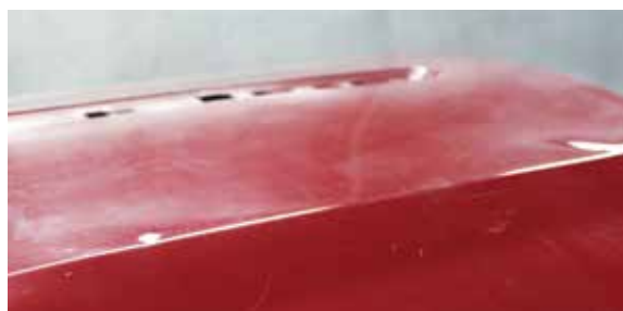
Corona treatment reduces the risk of imprinting on damp vehicles
