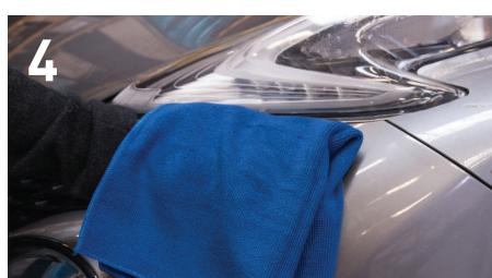
**EN** Lubricate the work surface with Norton Liquid Ice Detailer Spray. Use generously, and reapply if the clay starts to stick to the surface.
